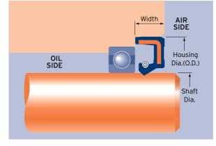
**BARNWELL REFERENCE A** - O.D. x shaft x width (ins) - material **A** - Shaft x O.D. x width (mm) - material
