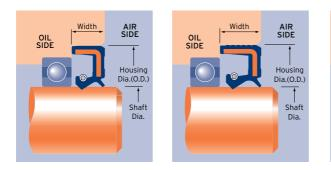
**BARNWELL REFERENCE AS** - O.D. x shaft x width (ins) - material **AS** - Shaft x O.D. x width (mm) - material
