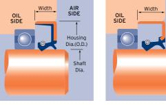
**BARNWELL REFERENCE BS** - O.D. x shaft x width (ins) - material **BS** - Shaft x O.D. x width (mm) - material Type S Totally encased built up single lip type
