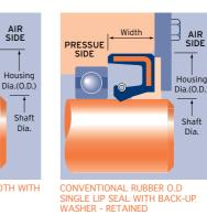
Pressure seals are available in Nitrile , Viton and PTFE in both inch and metric sizes.
