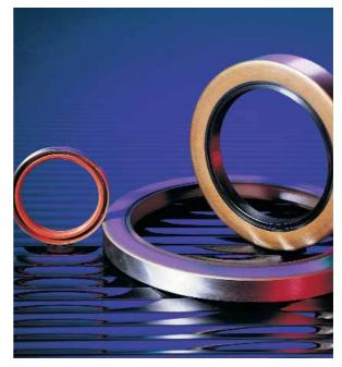
Similar construction to the 'B' type, metal O.D. (both ground and pressed & coated available), primary lip and additional dust/dirt lip (also called a wiper) moulded within the overall seal width but sometimes protruding outside the seal face. Usually referred to as "semi-dual" lip type they prevent the ingress of dust/dirt into the primary lip area. Available in inch and metric sizes in Nitrile, Viton, Silicone and Polyacrylic. Similar to "B" type range.
