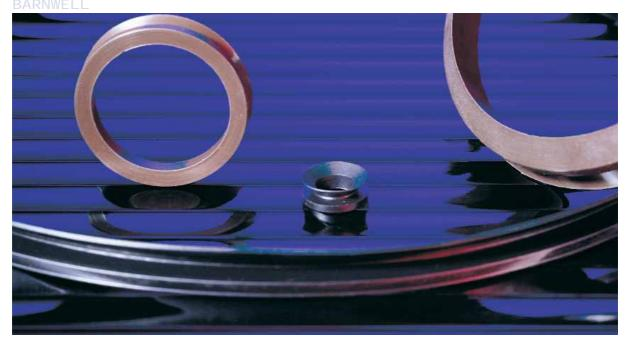
This all-rubber seal is generally a stretch fit onto a rotating shaft and unlike the previous RADIAL shaft seals described, this is an AXIAL seal. It can be used as a primary seal for grease or oil but is more commonly used as a secondary seal preventing the ingress of dirt, dust or water. Several styles are available, the more popular shown here.
