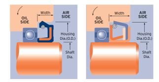
**BARNWELL REFERENCE EXT-R** - O.D. x shaft x width (ins) **EXT-L** - O.D. x shaft x width (ins) EXT-R - Shaft x O.D. x width (mm) EXT-L - Shaft x O.D. x width (mm)
