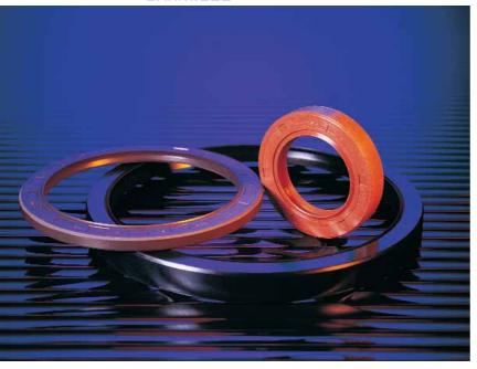
Similar construction to the 'A' Type - rubber O.D., with metal insert, primary lip and an additional dirt/dust lip (sometimes called a wiper) moulded within the overall seal width or alternatively protruding outside the seal face. Both types are usually referred to as "semi-dual" lip type, as the name suggests they help prevent the ingress of dust/dirt into the primary lip area. Available in inch and metric sizes in Nitrile, Viton, Silicone and Polyacrylic, similar to the 'A' type range.
