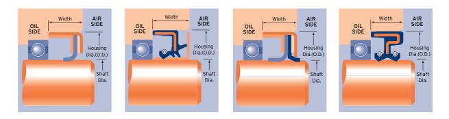
**BARNWELL REFERENCE** SP - O.D. x shaft x width (ins) SP - Shaft x O.D. x width (mm)
