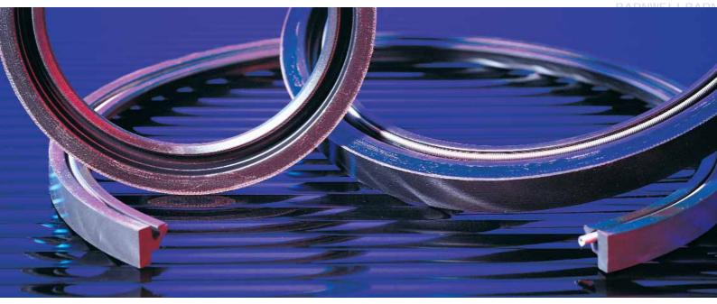
SPS Seals are solid rubber or rubber/reinforced fabric construction with a selection of garter springs to suit the application. Sizes are available to suit shafts from 3" upward, with no maximum limit. Widths and radial cross-sections generally conform to standard inch or metric sizes. SPS Seals can be supplied split or endless for "on-site" splitting with lubrication ports where required.
