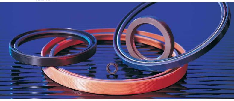
This is by far the most commonly used shaft seal design. The rubber O.D. permits replacement without damage to the housing bore, yet still retains the seal without the need for circlips, sealants or a retaining plate. Not suitable for high pressure applications.
