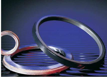
External seals are used generally for rotating hub applications. Seals, either rubber or metal I.D. are pressed onto the stationary shaft and seal against the bore. Housings must be kept smooth to prevent excessive wear as this diameter is greater than the normal running surface (shaft). The sprung lip version is the most popular but there are versions without springs as well as multi-grooved types sometimes found on agricultural equipment. Available in inch and metric, rubber or leather lips.
